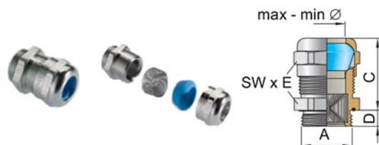
Figure 4-10 Example of a Blueglobe EMC cable gland
