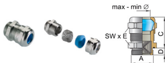
Figure 4-10 Example of a Blueglobe EMC cable gland
