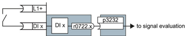
Figure 8-45 Load failure monitoring by means of a digital input
